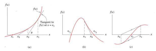
at  $x_1$  so that it intersects the *x*-axis at  $x_2$ . From the geometry of the figure, we may write
