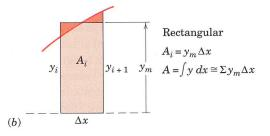
I. Rectangular [Figure (b)] The areas of the strips are taken to be rectangles, as shown by the representative strip whose height  $y_m$  is chosen visually so that the small cross-hatched areas are as nearly equal as possible. Thus, we form the sum  $\Sigma y_m$  of the effective heights and multiply by  $\Delta x$ . For a function known in analytical form, a value for  $y_m$  equal to that of the function at the midpoint  $x_i + \Delta x/2$  may be calculated and used in the summation.
