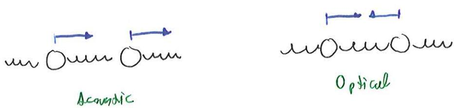
② In the diatomic basis case, the basis already has two distinct allowable frequencies  $\vec{q}$ , each one spreads into its own branch or band.
